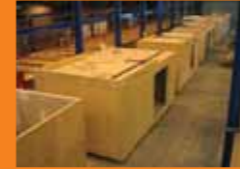
Volumetric pod production line
